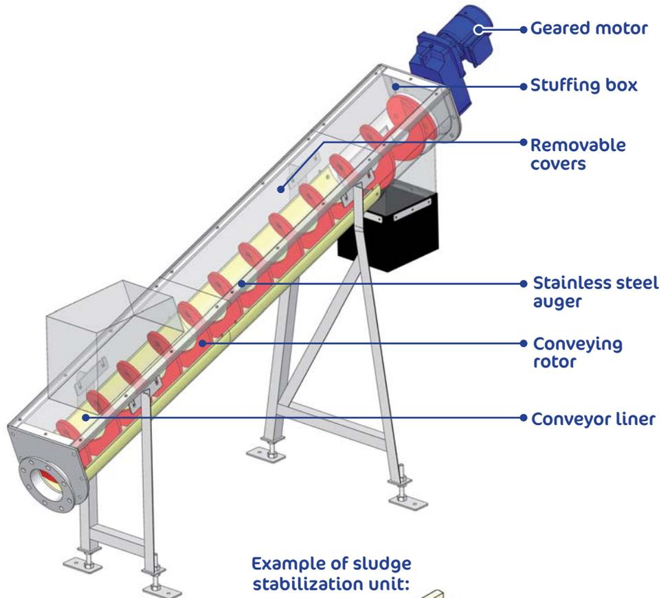
Example of sludge stabilization unit:
